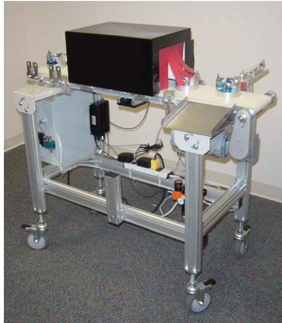
Figure 7. Fully automated system on 4 ft conveyor section, shown with acoustic chamber for testing parts.
