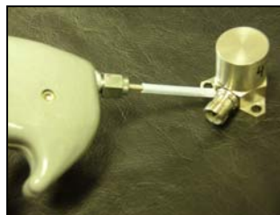
Figure 9C Leak Detection 'Sniff' Test on Weld Joint of a Hermetic Connector
