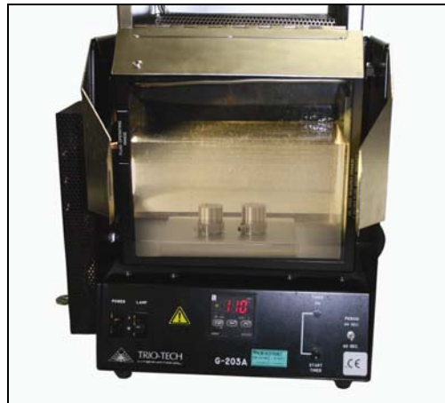
Figure 8 Gross Leak Test Apparatus TrioTech International G-203A Bubble Chamber
