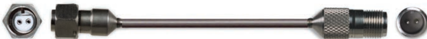
Model GN 2-socket 7/16-27 UNS-2B Plug 900 °F (482 °C) Model 013 2-Conductor Hardline Cable 1200 °F (650 °C) Model GP 2-pin 7/16-27 UNS-2A Jack
