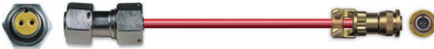
Model ET 2-socket, 7/16-27 UNS-2B Plug 400 °F (204 °C) Model 045 2-Conductor Softline PFA Cable 500 °F (260 °C) Model JD 2-pin Plug Mates to 2777A Series
