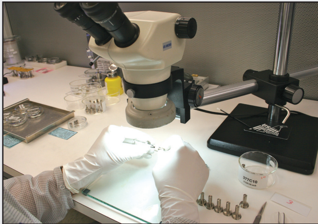
Photo 3: Final assembly of the mic capsules is done in a clean room environment. (Photo courtesy of PCB Piezotronics)
