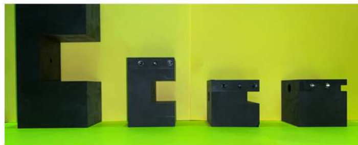
Structures with different sizes of square cavity ( a, a/2, a/4, a/8 )
