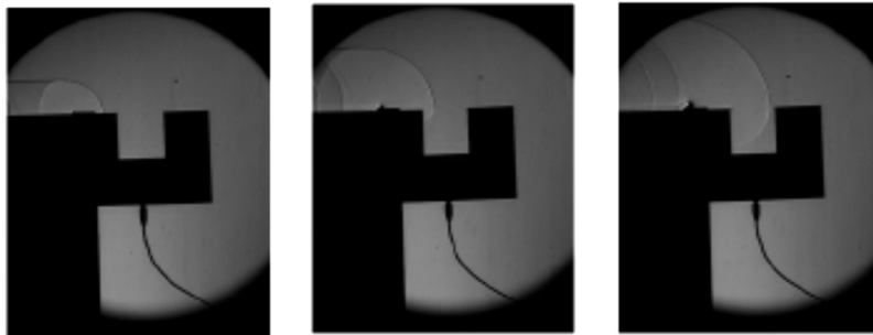
Pressure wave propagation inside the cavity.
