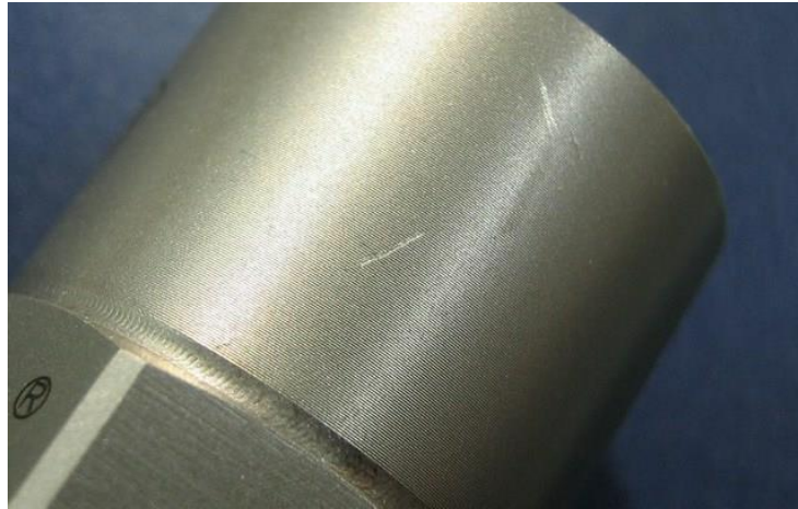
Figure 12 Unacceptable Scratches on Part Example
