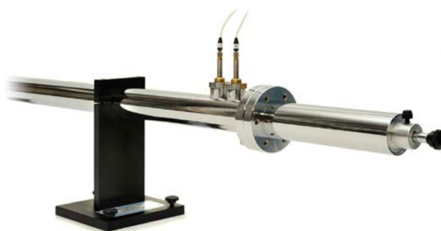
Flush Mounted Microphone Measurements in an Impedance Tube
