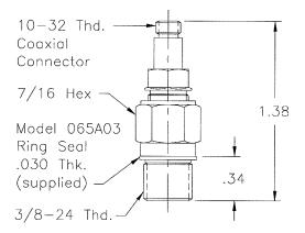
Series 102A10: Cryogenic Pressure Sensor
