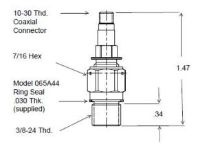
Series 102B10: Cryogenic Pressure Sensor
