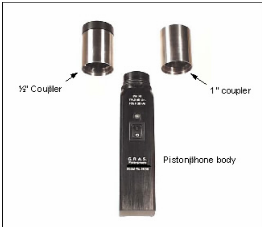
Fig. 8 1/2" coupler and 1" coupler
