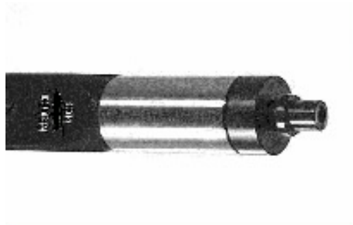
Fig. 7 1/4" Microphone adapter in 1/2" coupler
