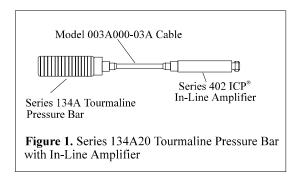
The Tourmaline Pressure Bars is a high-pressure, fast rise time, suppressed-resonance blast sensor ideal for single-shot, high-frequency measurements of incident or reflected shock wave pressures found in studies of plasma physics and hyper-sonics. Ranges up to 20,000 psi are available.
