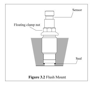
If thermal transients or diaphragm impingement are concerns, use the flush mount technique only when space or frequency response considerations preclude the use of the recess mount installation.
