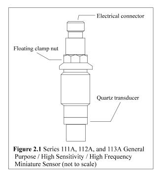
This rugged instrument measures transient or repetitive phenomena, relative to the initial or average level, over a wide amplitude and frequency range. It comfortably tolerates adverse environmental conditions. The sensor follows transient events up to a few percent of the system time constant, which, depending on the system, may be sufficient for static calibration by conventional methods. The sensor's internal design consists of a rigid, multi-plate, compression mode quartz element.
