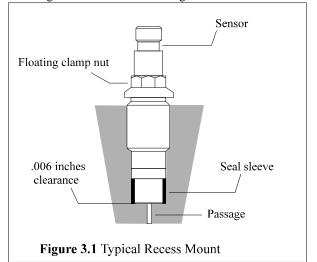
When using a recess mount, note that the length of the passage may limit the frequency range of the measurement. The effect the passage has is similar to that of an under-damped second order system, with the resonant frequency determined by passage length. The passage length thus limits pressure pulse rise time and may also cause passage ringing.
