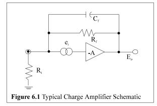
The feedback capacitor  $C_f$  comes into play only in the dynamic situation and its influence does not affect the steady-state situation. The voltage  $e_i$  is a DC offset voltage, usually very tiny (microvolts), that exists at the input gate of the MOSFET circuit. This minute leakage current exists in all real devices.
