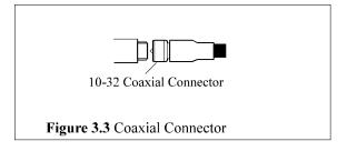
Plug the male connector on the cable into the mating female connector on the sensor. Then, holding the sensor stationary, secure the connector in place by tightening down the attached cable sleeve. See Figure 3.3.
