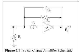
The feedback capacitor  $C_f$  comes into play only in the dynamic situation and its influence does not affect the steady-state situation. The voltage  $e_i$  is a DC offset voltage, usually very tiny (microvolts), that exists at the input gate of the MOSFET circuit. This minute leakage current exists in all real devices. As demonstrated in Equation 1, the steady-state (DC) output voltage  $E_o$  is:
