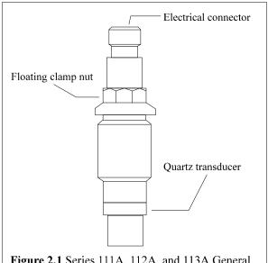
**Figure 2.1** Series 111A, 112A, and 113A General Purpose / High Sensitivity / High Frequency Miniature Sensor (not to scale)
