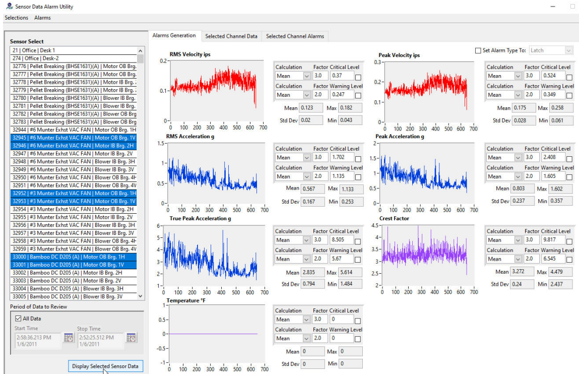
Figure 70 – Echo ® Alarm Generation Screen with multiple sensors selected
