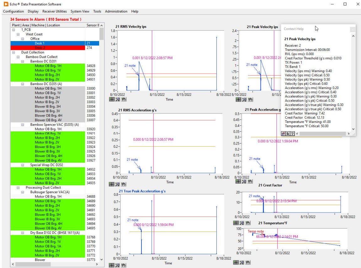
Figure 30 – PCB Echo® Main Screen showing status indications
