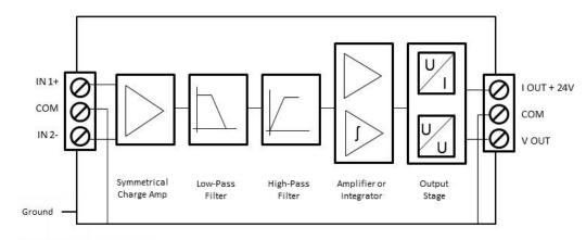
The amplifier converts the charge-based signal from a piezoelectric transducer into a current and voltage signal.
