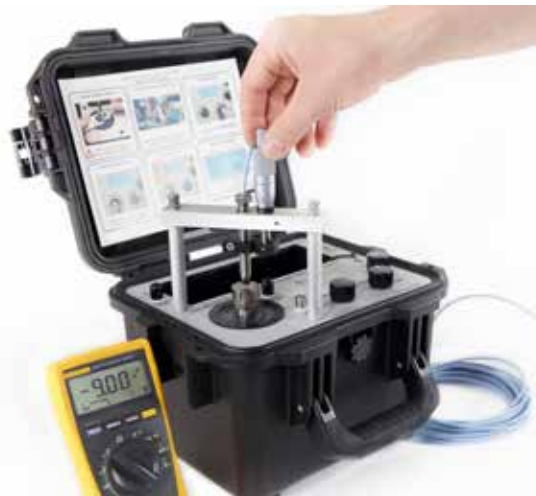
Technician adjusts position of proximity probe to correct for this error
