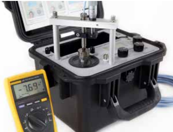
Incorrect cable length causes gap voltage to decrease
