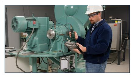
IMI Sensors has developed Model EX629A11A/006CC, a hazardous area-approved triaxial accelerometer to be used in route-based predictive machinery maintenance in hazardous environments for vibration monitoring. This new model utilizes a shear mode geometry ceramic piezoelectric element in an epoxy-sealed, stainless steel housing with an integral 6ft. polyurethane coiled cable and choice of terminating connector.
