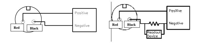
Figure 2 - wiring: loop powered
