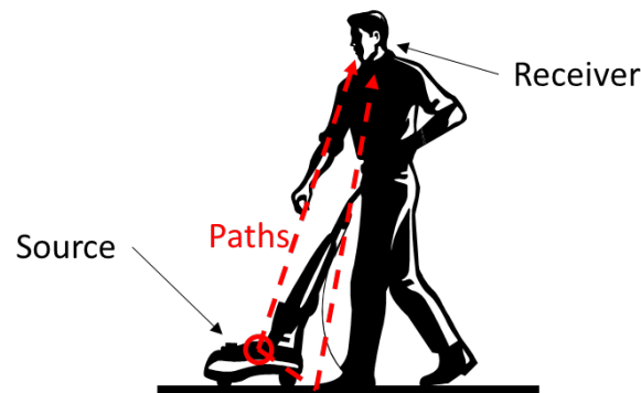
Figure 1. Schematic of a source-path-receiver paradigm for a vacuum cleaner. Notice that there can be multiple paths that the sound can travel to reach the receiver. Here both the direct and reflected paths are depicted.
