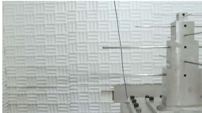
The picture to the above left shows the PCB microphone (Model Y378A13, S/N U103169) set up. The picture to the right visually shows the first resonance of the bottom rod (15.25 in).
