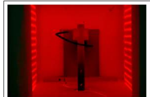
Figure 1: High-temperature accelerometer during vibration at 1400 °F (760 °C).
