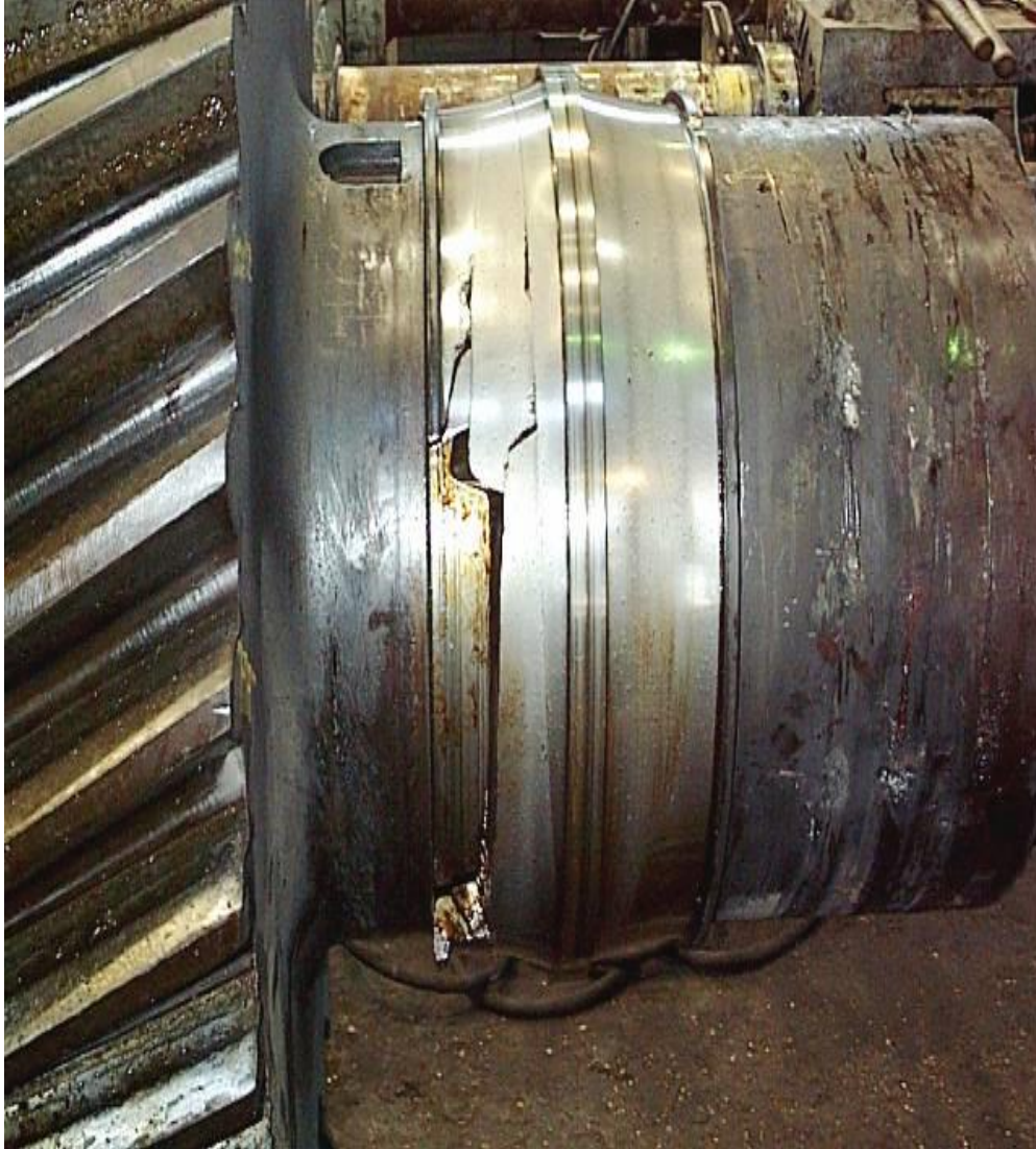
Figure 4 Picture of defective bearing from the hot mill pinion stand gearbox
