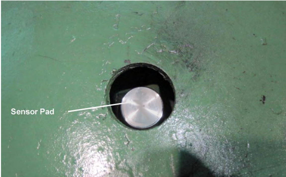
Figure 6 Mounting Pad attached to flat spot under the end bell
