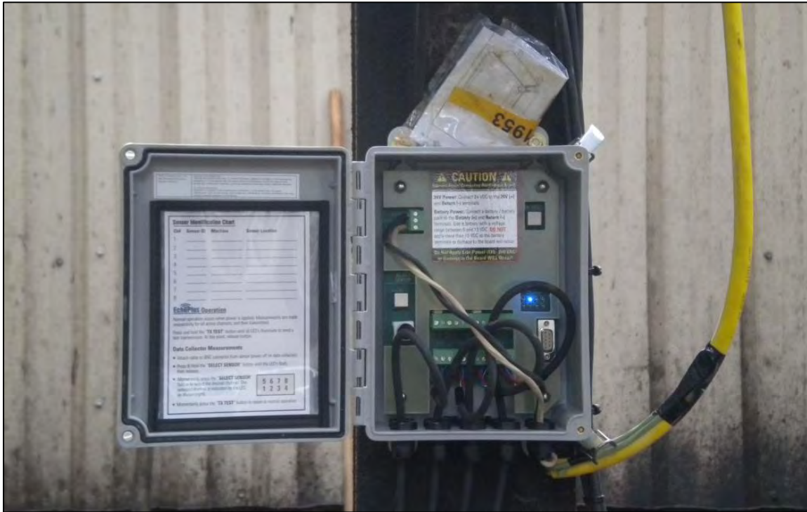
Figure 3 – EchoPlus® Measuring One of Eight Connected Accelerometers
