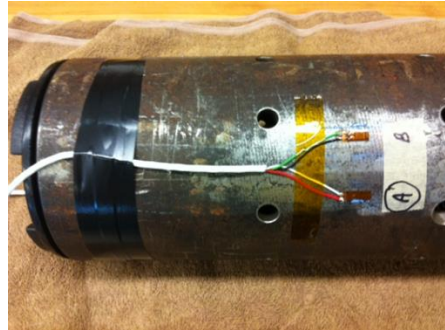
Figure 7: 1000 Ohm Karma Gage Pairs Cabled with Vishay 430 FST Cable
