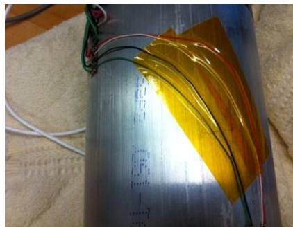
Figure 6: Transitional wiring to 4-Wire Shielded Cable
