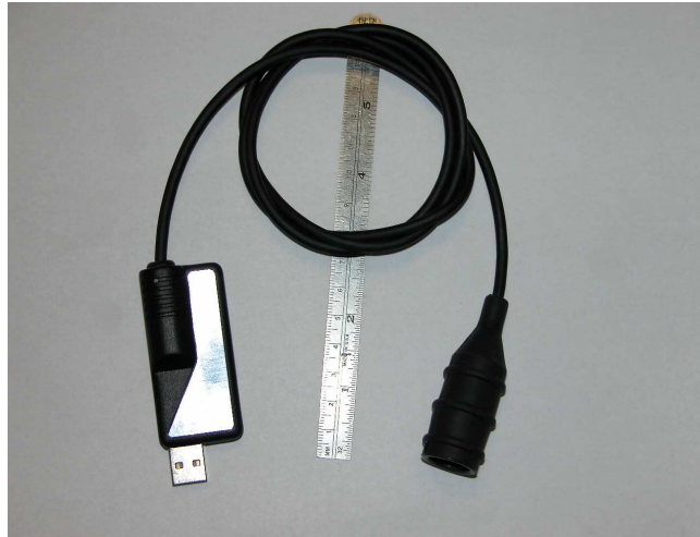
Figure 8 – IMI Model 070A82 USB Programmer
