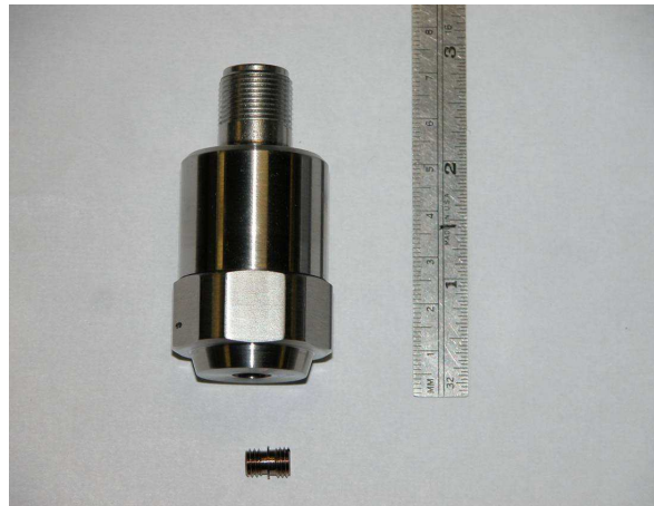
Figure 7 – IMI Model 649A01 Reciprocating Machinery Protector
