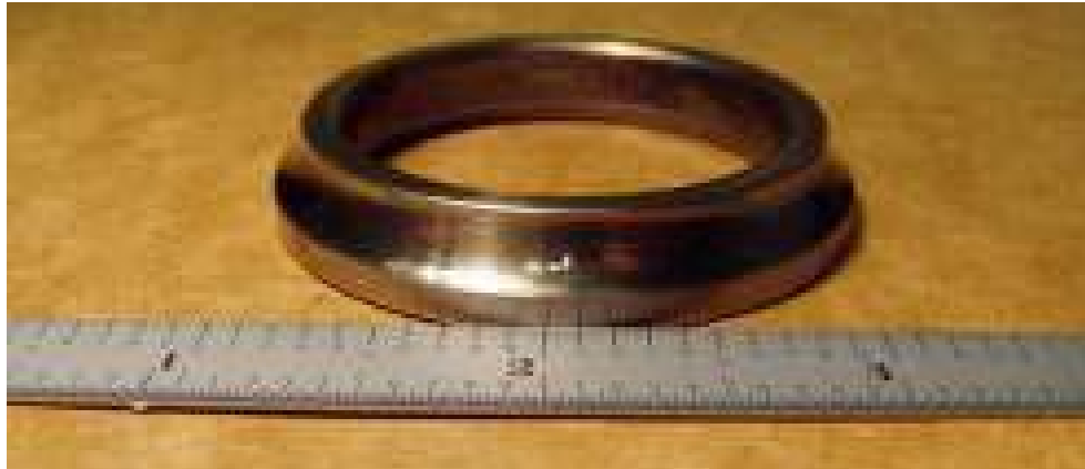
Figure 13 Spalled Bearing of the Pinion Stand Gearbox detected by BFD
