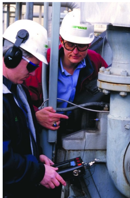
Figure 8: Data collection using a walk around data collector with a magnetically mounted high frequency ICP ® accelerometer (Photo courtesy of Praxair)
