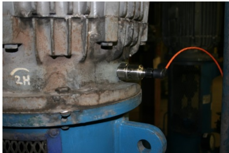
Figure 9: Permanently mounted ICP® accelerometer on a motor.
