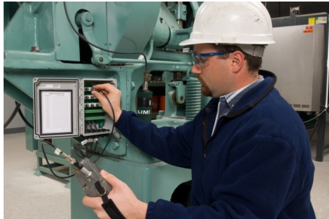
Figure 10: Data collection using a walk around data collector, permanently mounted ICP® accelerometers, and an IMI junction box.
