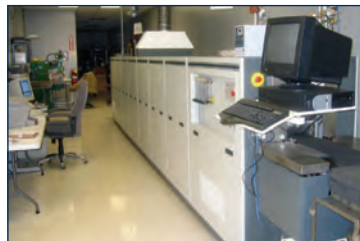
Electrical connectors with glass-to-metal fused hermetic sealing are processed in a conveyor furnace
