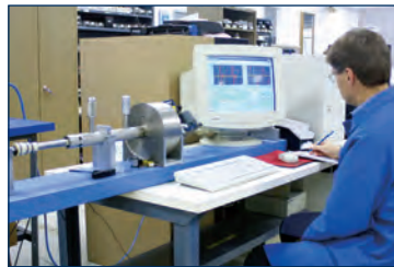
High-amplitude Hopkinson Bar Linearity & zero shift tests with exposures to impact shocks of more than 100k g
