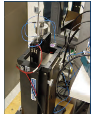
Low-frequency Accelerometer Calibrator 6" (152 mm) stroke shaker provides displacement for calibrations to 0.5 Hz
