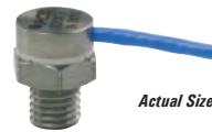
Model 3501A1220KG Single Axis ■ 3 gm ■ Titanium housing ■ Integral copper cable (10 ft/3.1m) ■ 1/4-28 Thread
