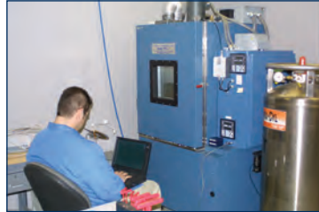
Environmental Stress Chamber HALT, HASS & other thermal chamber tests on prototypes and production output
