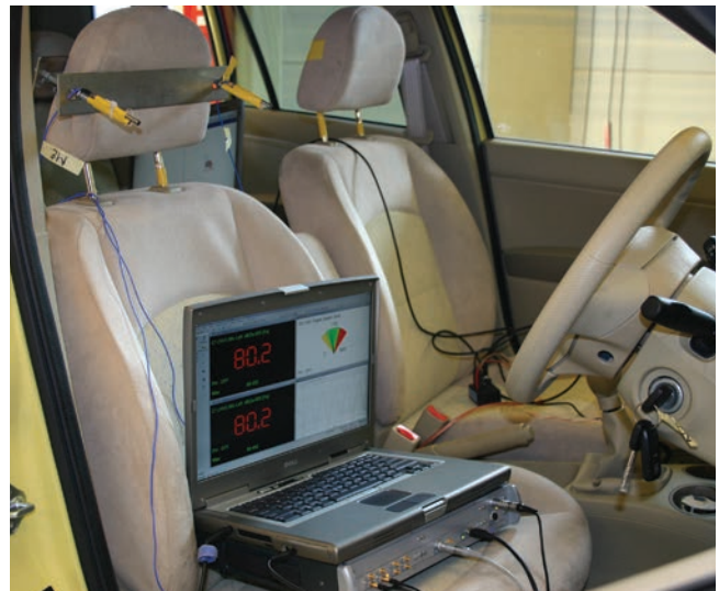
Cabin Noise Measurements for Rider Comfort
