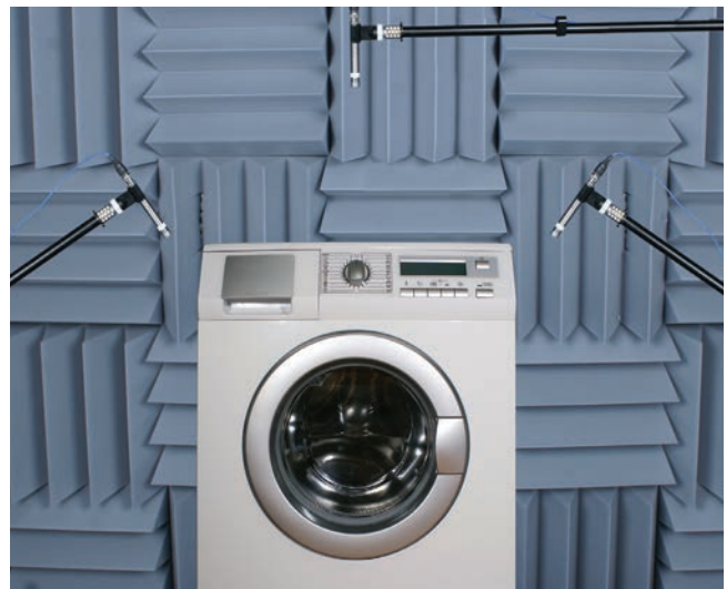
Sound Source Location for Noise Reduction
