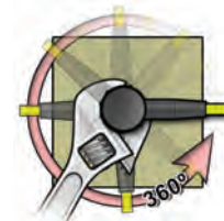
Using the 360° capabilities of the Swiveler®, the cable is positioned into desired orientation & temporarily hand tightened. Using a wrench, the hex nut is tightened to the recommended torque while holding the cable or connector in the desired location.
