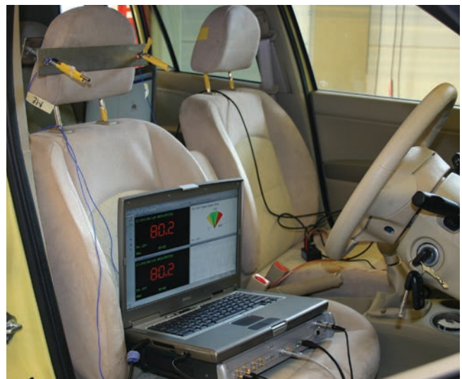
Cabin Noise Measurements for Rider Comfort
