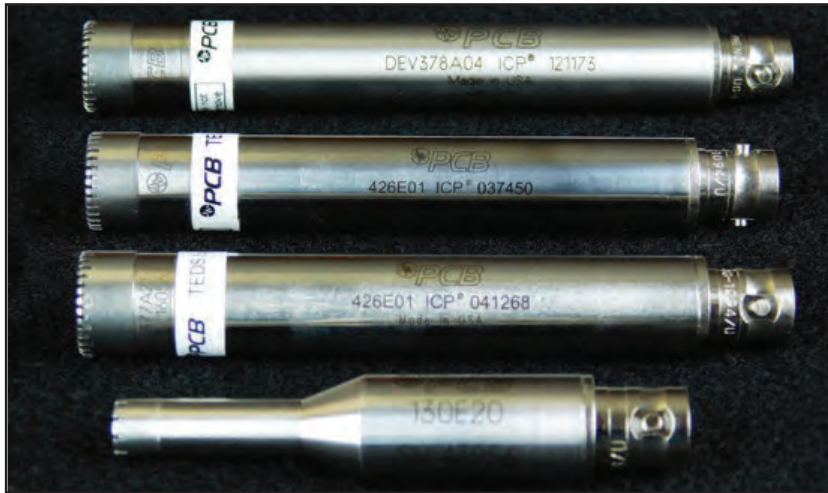
Photo 2: The four PCB Piezotronics microphones that I tested vary in size. (Photo courtesy of Cynthia Wenslow)
