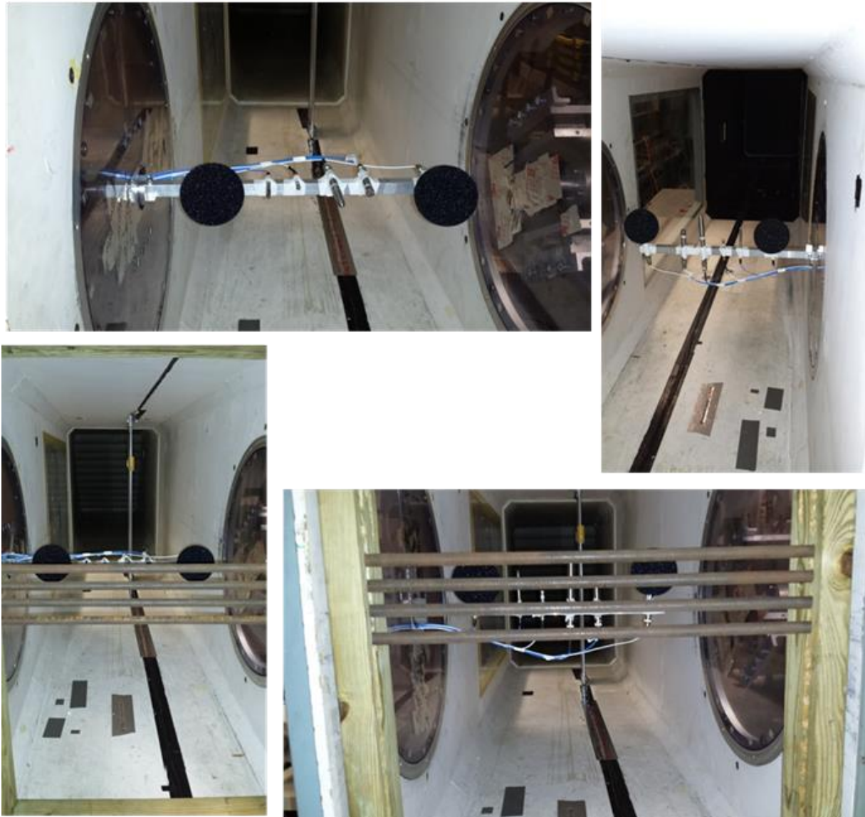
Figure 2. Microphones shown mounted in the wind tunnel in the head-on (left) and parallel (right) orientation, with (lower) and without (upper) the turbulence generator. Flow direction is into the page.
