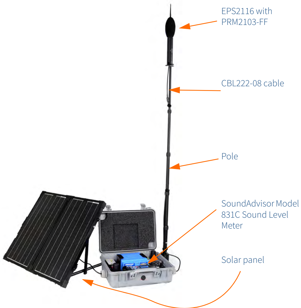
FIGURE 1-3 Remote Noise Monitoring System (SoundAdvisor NMS044)
