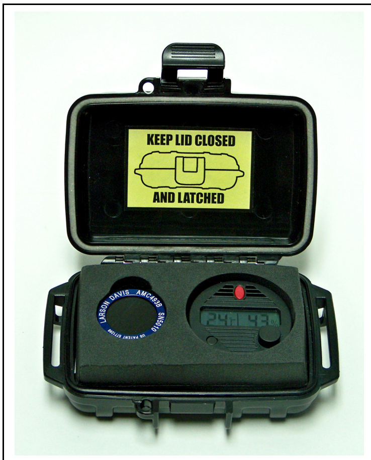
FIGURE 4-1 CCS043 Case with AMC493B and Digital Hygrometer/Temperature Meter
