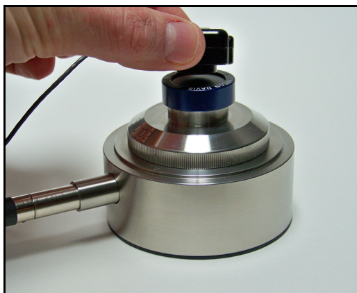
FIGURE 3-2 Placement of the bone vibrator on the AMC493B Artificial Mastoid
