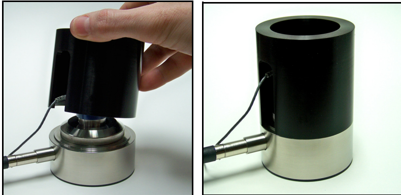
FIGURE 3-3 Placing the retaining ring on the coupler
