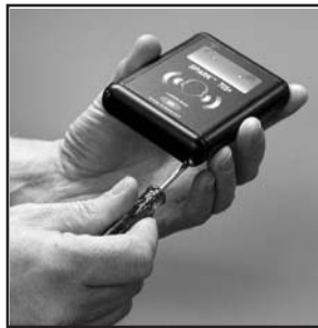
Figure 1-14 Replacing the battery door
