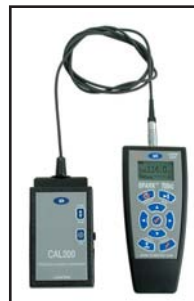
Figure 2-1 Calibrating the Spark ™ -ATEX
