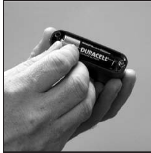
Figure 1-13 Replacing the battery
