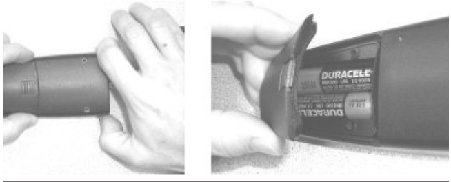
Figure 1-8 Opening the battery door
