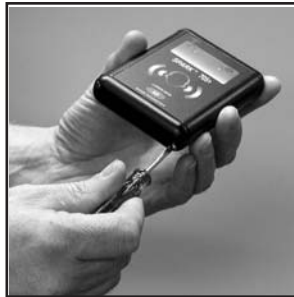
Figure 1-11 Removing the battery door
