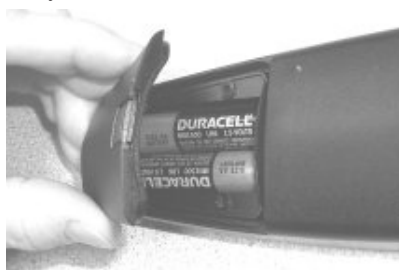
Figure 1-9 Re-inserting the battery door
