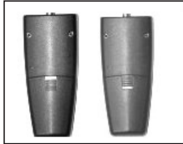
Figure 1-7 Moving the battery door sliding tab
