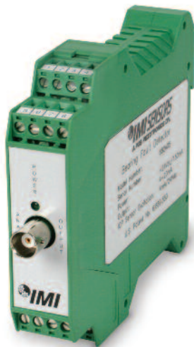
Model 682A05 Bearing Fault Detector *(US Patent Number 6,889,553)
