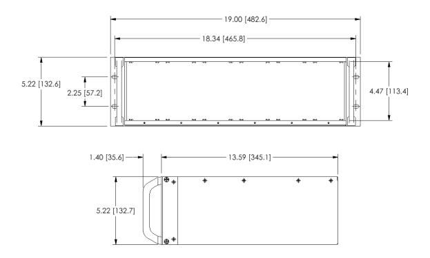
The Endevco Model 4948A is a 19 inch rack that houses up to 6 signal conditioner units of the Endevco Model 2775C or 6634D. The front end of the rack provides access and guidance by means of card guides. The rear end of the rack is completely open allowing the user to access the rear connectors of the 2775C or 6634D.
