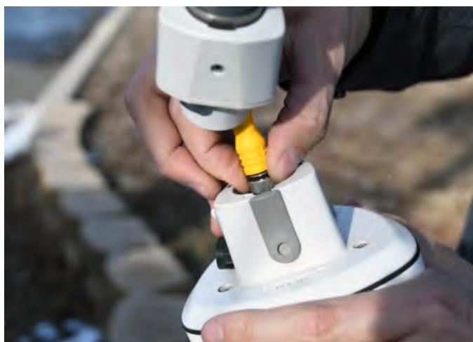
FIGURE 4-17 Feed CBL229-20 Through Weather Arm
