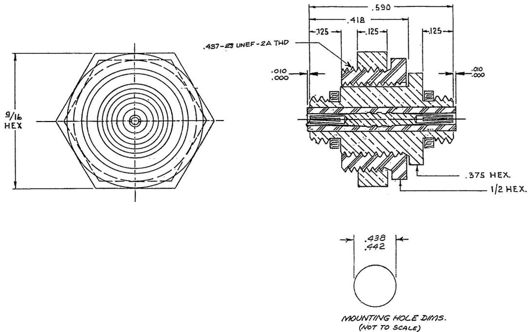
Feed-thru bulkhead microdot connector.
