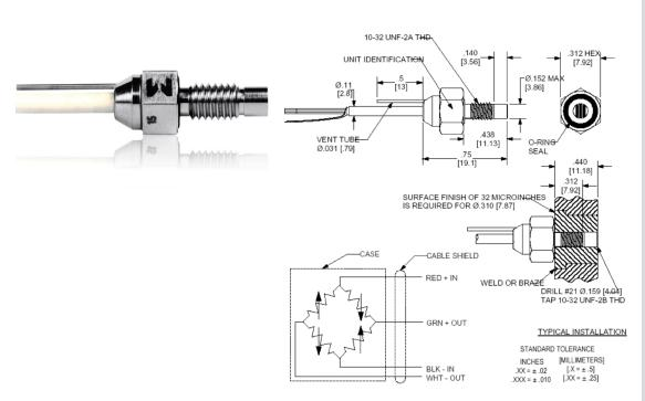
Model 8510B is a rugged, miniature, high sensitivity piezoresistive pressure transducer. It has a 10-32 mounting thread, 0.15 inch (3.8 mm) face diameter and is available in ranges from 1 psi to 2000 psi. Low pressure ranges are shown on this sheet. Its high sensitivity combined with high resonance makes it ideal for measuring dynamic pressure.
