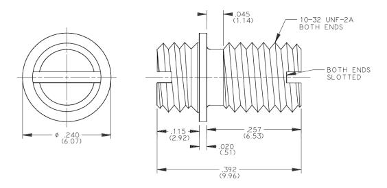
Mounting stud with slotted head for use with accelerometers with a 10-32 thread.
