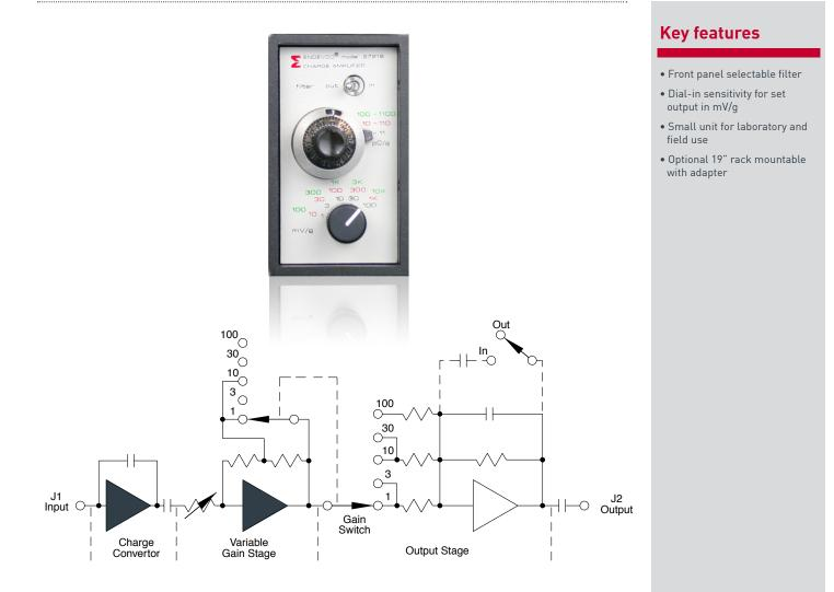
The Endevco<sup>®</sup> model 2721B is a charge amplifier for use with piezoelectric transducers with resistance as low as  $1k\Omega$ . Its small size and  $\pm 15$  VDC operation are suited to laboratory and field use. The output voltage of the amplifier is proportional to the charge at the input.
